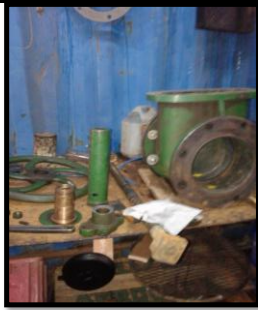
Válvula AGUA 8 " SALIDA BY PASS
